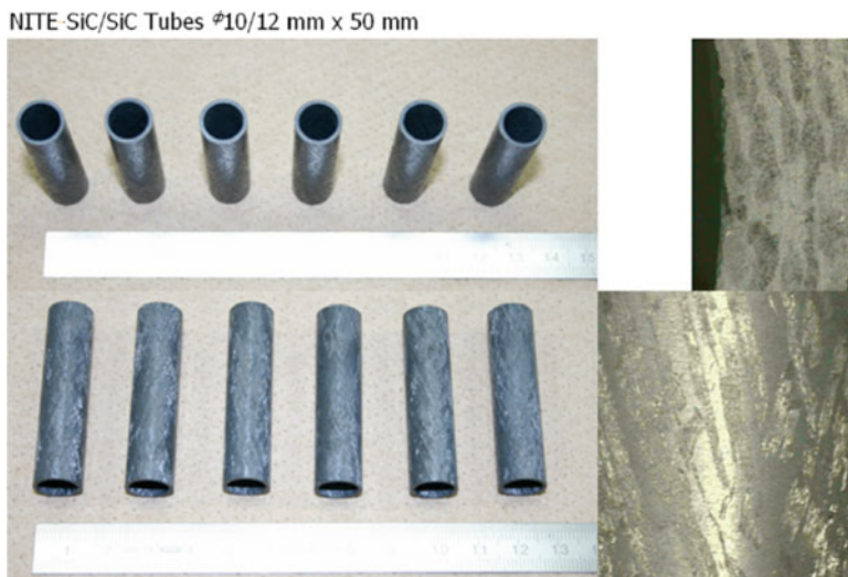
Fig. 9.11 SiC/SiC composite tubes made by third generation NITE method. Reproduced with permission from Katoh [418]. Copyright Elsevier
