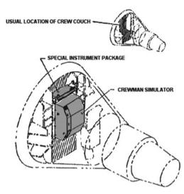
A schematic of the MA-4 capsule, showing the location of the crewman simulator. (Illustration: NASA)
