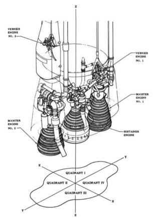
This schematic drawing shows the configuration of the five engines used on the Atlas rocket. (Photo: NASA)
