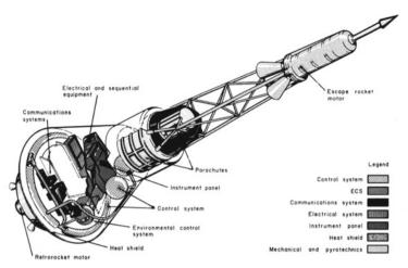
The Mercury capsule and escape tower. (Diagram: NASA)
