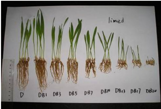
Fig. 2.6 Barley root elongation test. Phytotoxicity increases from left to right dependent on the used additive mixture
