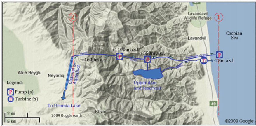
Fig. 19 Schematic layout of transferring sea water over Alborz coastal mountains
