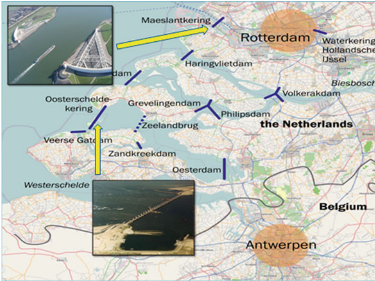
Fig. 4 Dutch Delta Works Project, a comprehensive flood control system featuring a coastal spine with conventional dikes as well as flood gates
