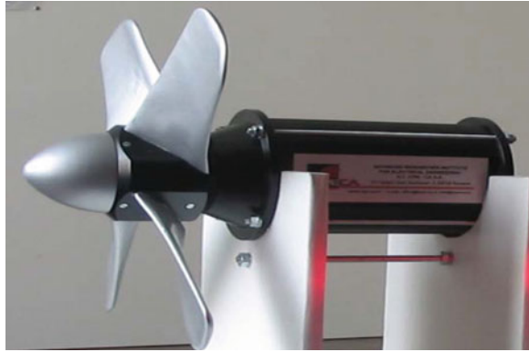
Fig. 4 Hydraulic turbine rotor directly coupled with the submersible electric generator
