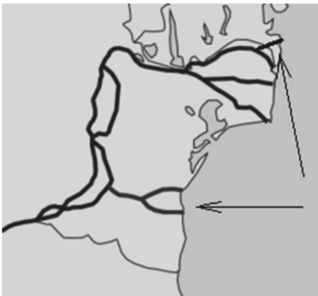
Fig. 13.5 Artificial navigational channels of the Danube river. Arrows point to the Ukrainian ( upper ) and Romanian channels
