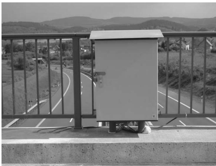
9.11 Measuring unit of exposure tests within the splash water zone of a highway in Germany
