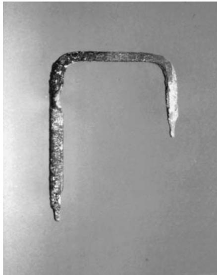
9.5 Corroded rebar from a 4 year old building in a hot, salty environment
