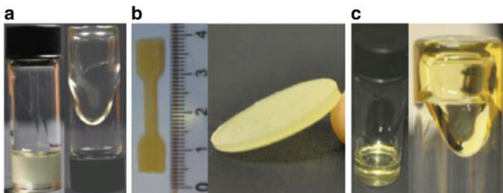
Fig. 12 Photographs of (a) DAT–PPO–2200–DAT, (b) Thy–PPO–2200–Thy, and (c) a stoichiometric mixture of Thy–PPO–2200–Thy and DAT–PPO–2200–DAT free matrix chains. Reprinted with permission from [32]. Copyright 2012 American Chemical Society
