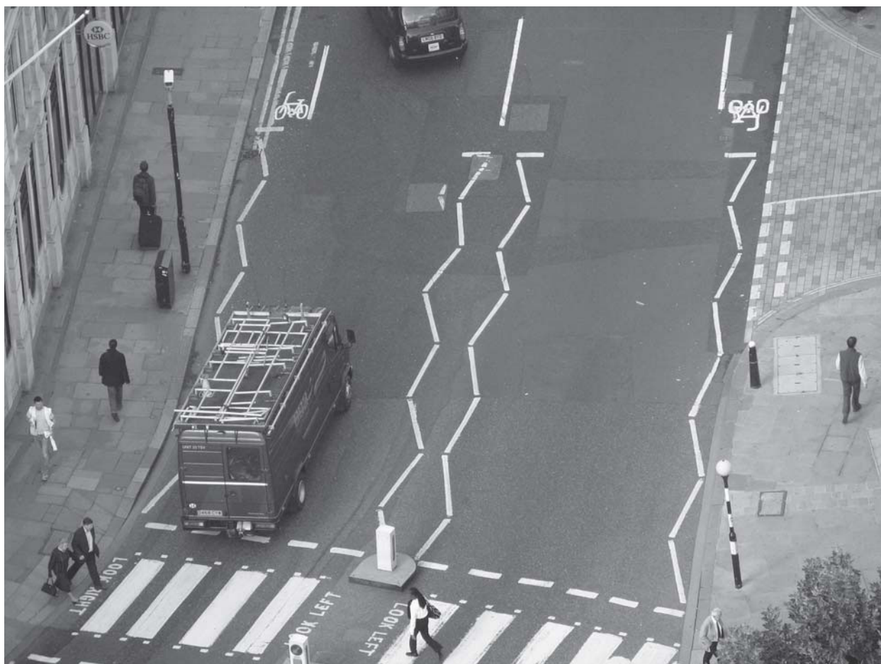
Figure 5.3 To ensure that pedestrians' view of oncoming traffic is not obscured, drivers in the United Kingdom are not allowed to park in areas marked with zigzag lines, one of many types of built environment interventions available to protect pedestrians and bicyclists (photo: Wikimedia Commons, courtesy of Benjamin D. Esham).
