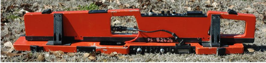
Fig. 1 Apparent soil electrical conductivity ( EC_a ) is often determined using an EM38. Shown above is a similar unit (EM38-DD, Geonics, Mississauga, Ontario, Canada) designed to collect both horizontal (effective measuring depth is approximately 75 cm) and vertical (effective measuring depth is approximately 150 cm) (McNeill 1980)
