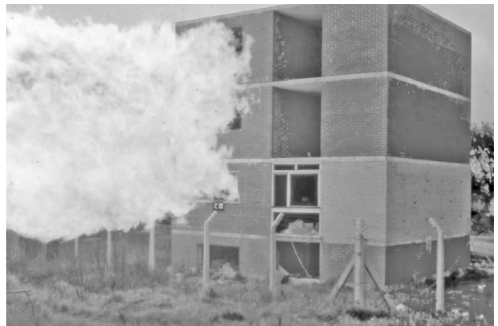
Figure 33 Explosion testing of masonry structure
