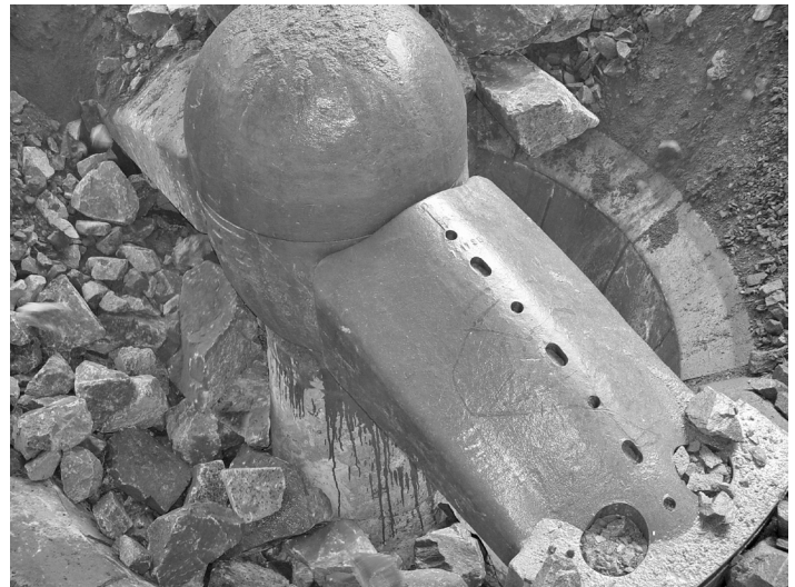
Figure 3 Direct feed of stone into a gyrator crusher (courtesy of QMJ Publishing Ltd)
