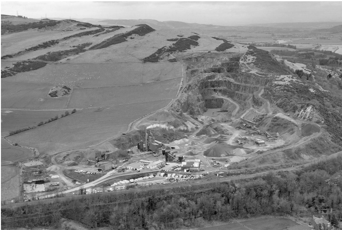
Figure 18 Aerial view of an igneous rock quarry (courtesy of Ennstone Thistle Ltd)
