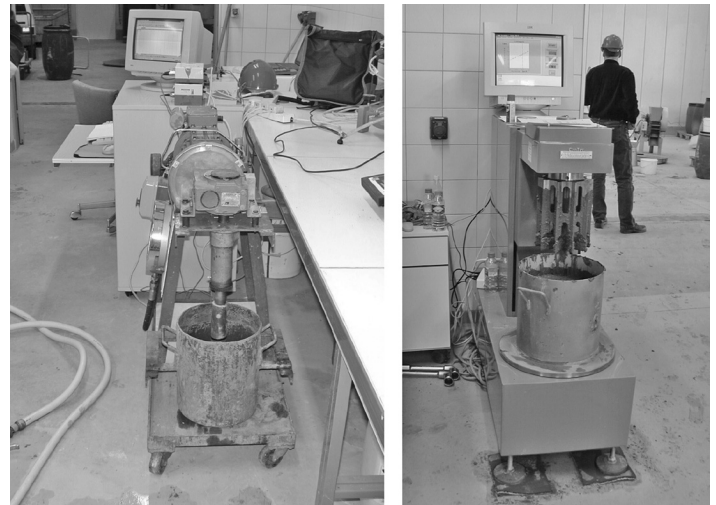
Figure 13 Two-point workability apparatus and BML rheometer
