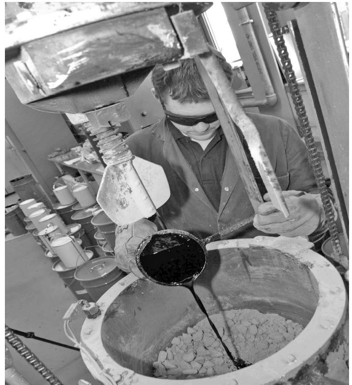
Figure 4 Laboratory production of asphalt mixture (courtesy of Shell Bitumen)
