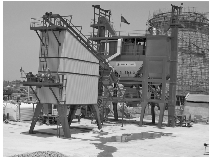
Figure 9 Conventional asphalt batch plant (courtesy of ACP Titan Overseas Ltd)
