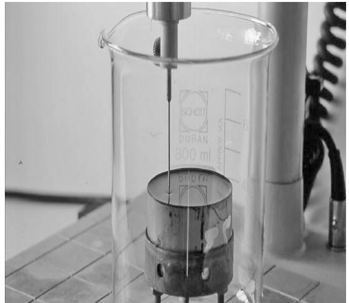
Figure 2 The penetration test for bitumen (courtesy of Shell Bitumen)
