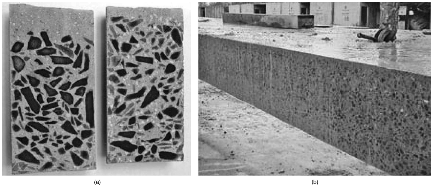
Figure 9 The effect of vibration on concrete segregation: (a) over-vibrated concrete; and (b) self-compacting concrete placed without vibration (C. Ozyildirim, Consolidation concerns continue, Concrete International, 2005)
