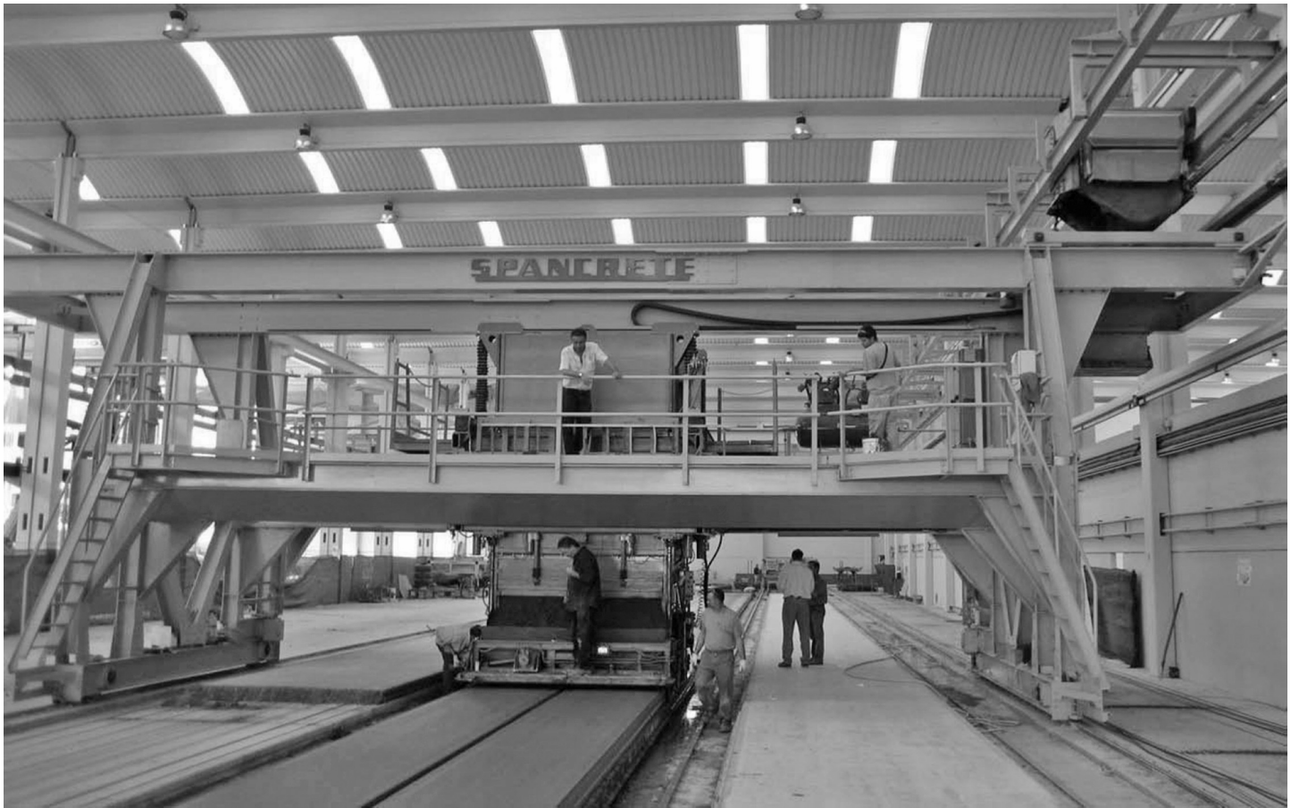
Figure 6 Production of Spancrete ® hollowcore plank (courtesy of Kim Walker, Spancrete Group, Inc., USA)
