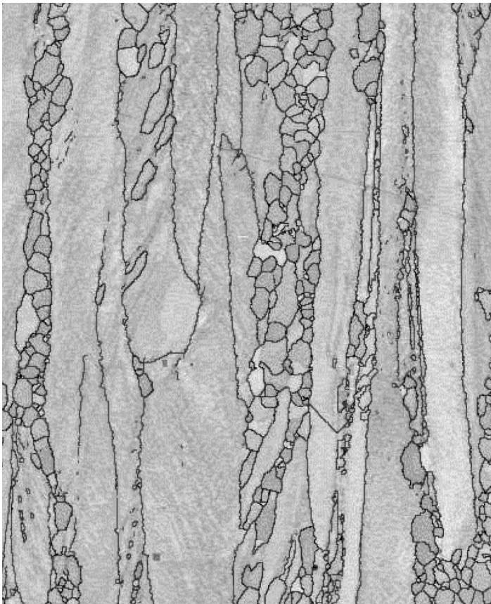
Figure 14 Iron aluminide: Polycrystalline grain structure. The electron back-scattered diffraction image shows the orientation of the grains after casting, deformation and heat treatment. (Image by Jane Blackford, University of Edinburgh)
