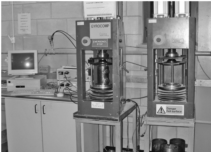
Figure 6 Gyratory compactors (courtesy of Shell Bitumen)
