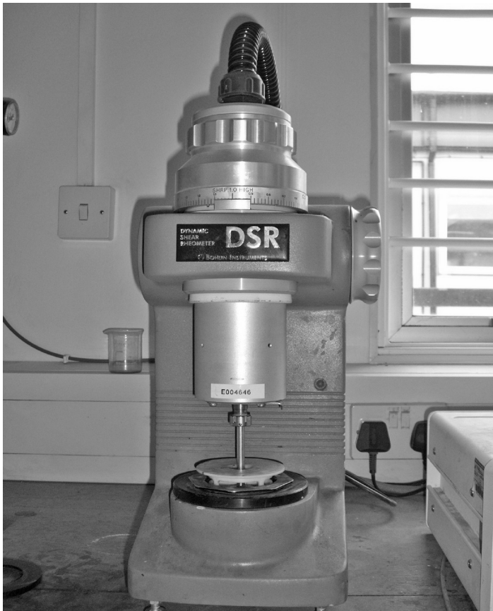
Figure 3 A dynamic shear rheometer (courtesy of Lafarge Aggregates Ltd)
