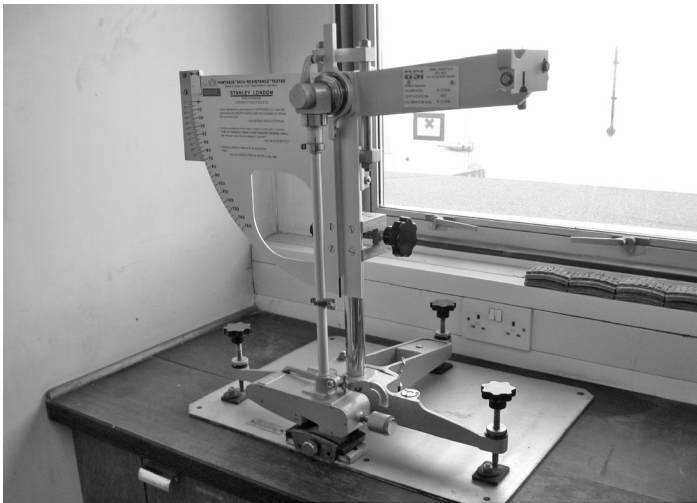
Figure 1 Polished stone value apparatus (courtesy of Lafarge Aggregates Ltd)
