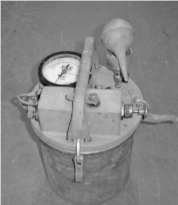
Figure 14 Pressure method to measure air content
