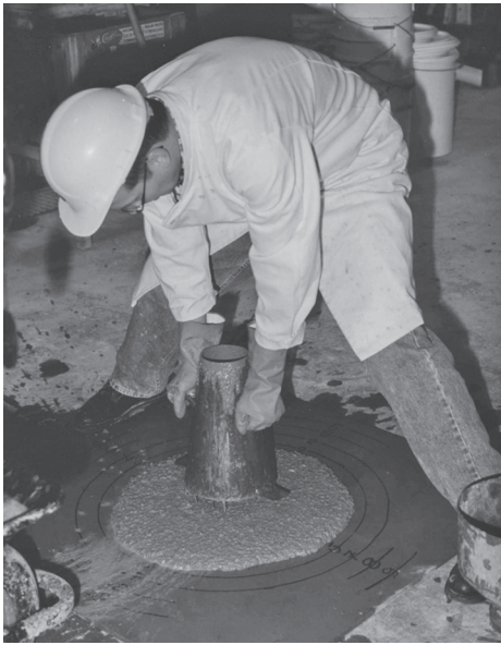
Figure 6 Slump flow test and T_{500} time
