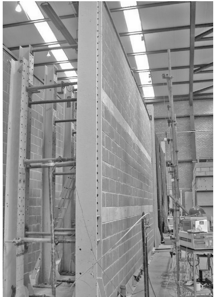
Figure 5 WI beam construction test wall
