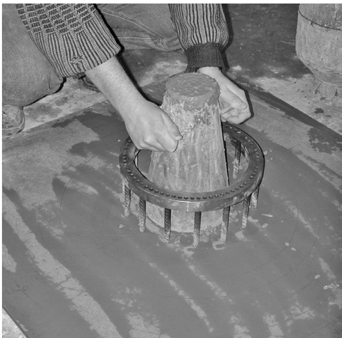
Figure 9. J-ring combined to slump cone
