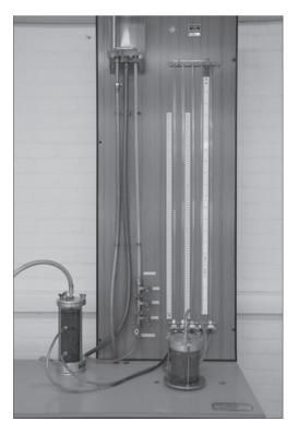
Fig. 5.1 Laboratory permeameters.
