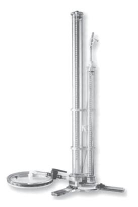
Fig. 5.8 A tension infiltrometer. Reproduced with permission of Soil Measurement Systems.
