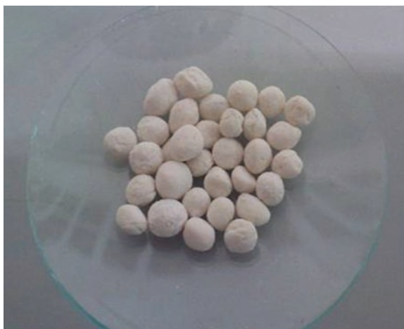
Fig. 4.8 Hand-made spheres of Sipernat 320-based SiO 2 : the diameter of each sphere is approximatively 0.5 cm
