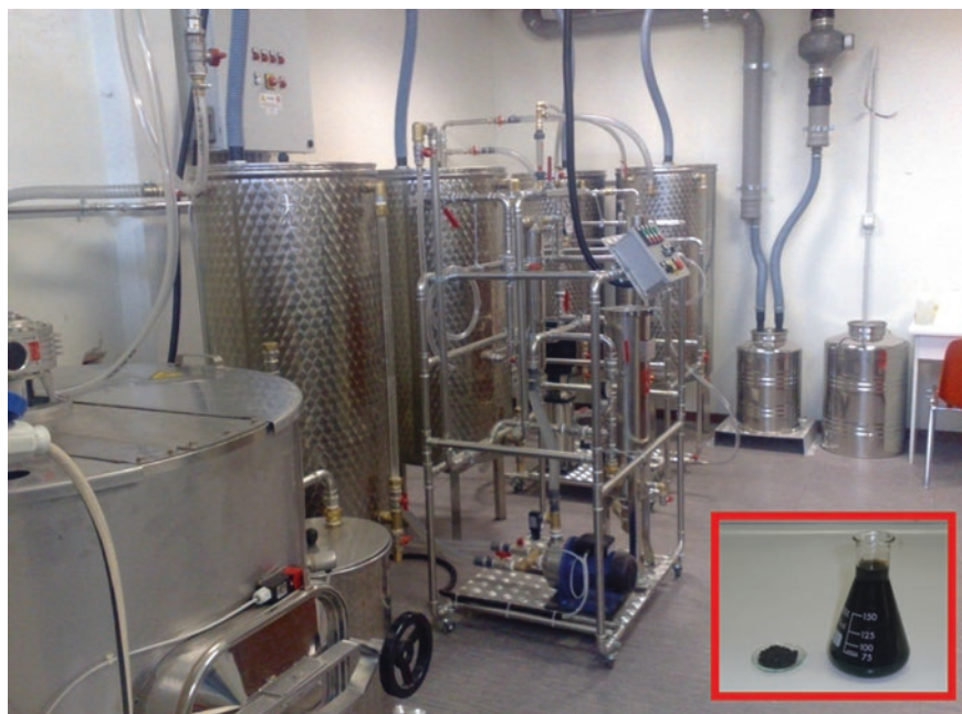
Fig. 1.3 Pilot plant for SBO isolation. Inset: SBO powder and its concentrated water solution
