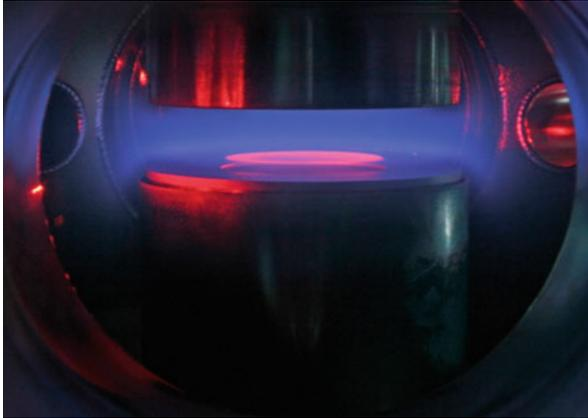
**Fig. 6.2** Horizontal dust plasma crystal formed above the lower electrode of a GEC RF cell. Dust particles float at an equilibrium height where the gravitational force is balanced by electrostatic force due to external electric field. The confinement in the horizontal direction is provided by an inwardly directed force created by a ‘cut-out’ plate placed on the lower electrode. Image source: Center for Astrophysics, Space Physics, and Engineering Research, Waco, TX
