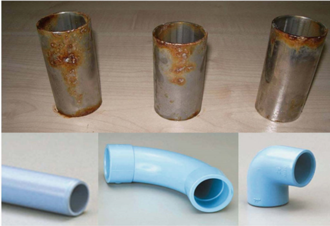
Fig. 3.2 Corrosion damages on different materials for food processing systems. Stainless steel is widely used; on the other hand, corrosion processes can be notably reduced by means of plastic materials such as chlorinated polyvinyl chloride (C-PVC)
