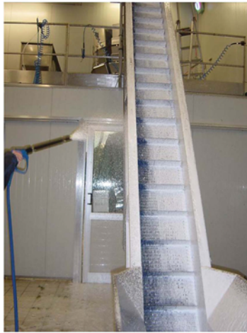
Fig. 3.5 Conveyor belts may be easily contaminated by microorganisms, especially when porous or fibrous materials have been used in their construction. The final sanitisation may be very helpful
