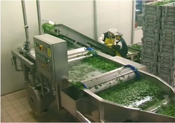
Fig. 3.1 The chemical composition of food-contact materials may offer several contamination possibilities, including microbial contamination. Basically, food-contact surfaces are correlated to containers and objects for processing equipments such as washing machinery for fresh vegetables
