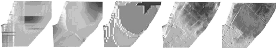
Fig. 2.6: DEMs obtained using different data sources and interpolation methods. From left to right: raster and TIN (Triangular Irregular Network) DEMs produced by the Swiss Federal Office of Topography, a raster DEM produced by IGUL (Institute of Geography of the University of Lausanne, Switzerland) and two raster DEMs based respectively on photogrammetry of aerial photographs and analysis of airborne laser measurements (Metzger, 2002). Spatial discontinuities related to roadways present in the area can be distinguished only on the last DEM (adapted from Metzger, 2002).
