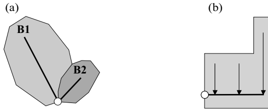
Fig. 9.8: Hydrological configurations for which the rational method cannot be applied without precautions (see Appendix 9.6.2). a) The case of a basin made up of a rural basin (B1) with a slow response producing little runoff and a small but highly productive urban basin (B2) with a fast response. b) The case of a basin with a hydrological irregularity.
