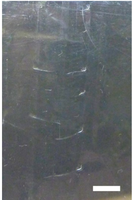
Fig. 7.4 Pigment bands in a plastic film. Observation conditions: optical microscope, objective 5×, transmitted white light
