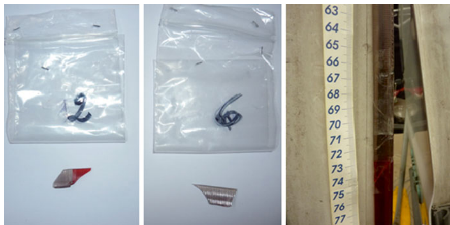
Fig. 6.2 Plastic items found in the vicinity of the wall where the broken tomb was. The picture on the right shows the perfect correspondence of the items with the broken part of the tail reflector
