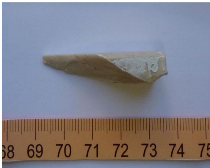
Fig. 4.2 A paint smear on a piece of marble, allegedly left by a van hitting a wall
