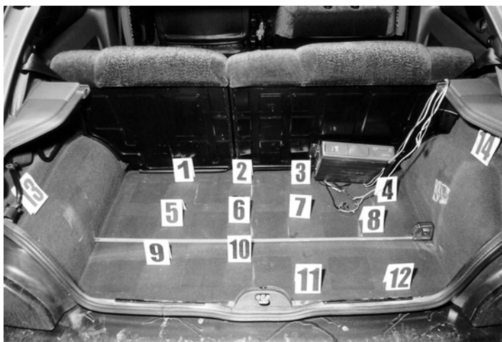
Fig. 4.1 The trunk of this car was divided into 14 areas, each one about 20×20 cm 2 in size, which were sampled by repeatedly using 10×10 cm 2 pieces of adhesive tape. Reprinted from [21], copyright 2004, with permission from Elsevier
