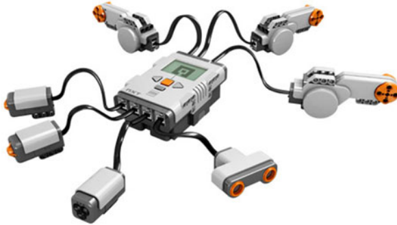
Figure 3.4 – The NXT programmable brick along with the sensor and actuators shipped with the LEGO Mindstorms NXT 2.0 Kit.
