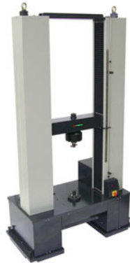
Figure 1.2 – Professional tensile test equipment. Zwick 314 Series 11 .
