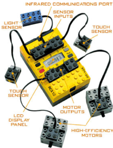
Figure 3.3 – The Robotic Command eXplorer (RCX) programmable brick along with the sensor and actuators shipped with the LEGO Mindstorms Robotics Invention Kit.
