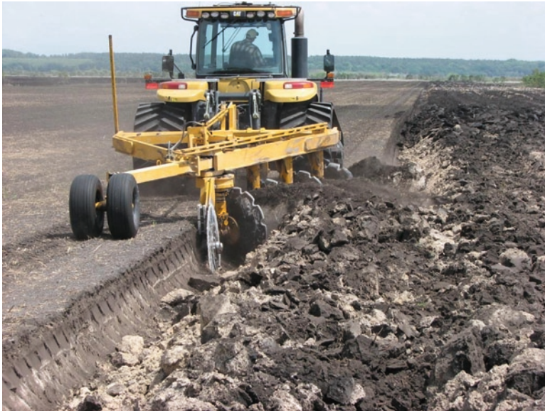
Fig. 6.5 A tractor pulls a special plow that places potentially contaminated soil deep below the surface as part of a soil inversion project. Credit SJRWMD
