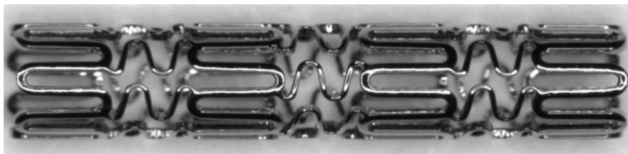
Fig. 9.2 Brightfield microscopy image of drug-eluting stent (8-mm long Cordis Cypher stent)
