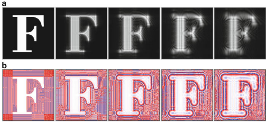
Fig. 4.5 An example of numerical diffraction by angular spectrum method, using the same parameters as in Fig. 4.3. (a) Amplitude images and (b) phase images
