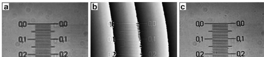
Fig. 12.1 Example of refocusing capability with a digital holography microscope on a metric scale (100 divisions/mm), illuminated with a LED. (a) Intensity of the defocus, (b) phase of the defocus image, and (c) computer-refocused image. The refocus distance is 80 \mu\text{m} . (Reprinted from [1] by permission of OSA)
