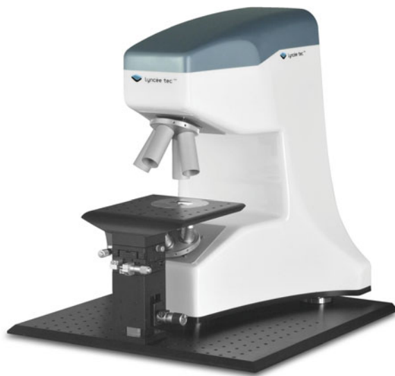
Fig. 11.9 Lyncée Tec DHM T1000 digital holographic microscope. (Courtesy of Dr. Yves Emery, Lyncée Tec SA)
