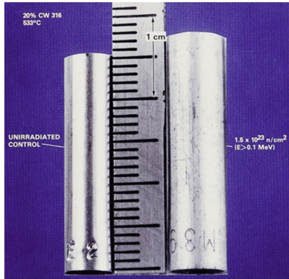
Fig. 2.1 Stainless rods before (left) and after (right) irradiation [2]. The irradiated sample shows swelling caused by an accumulation of gas in the lattice interstitials
