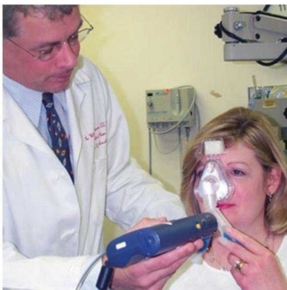
Fig. 4.2 Image of breath testing using electronic nose composed of GNPs (Credit Image courtesy by Emily Anthes, http://www.scientificamerican.com/article/electronic-noses-could-make-diseases-something-to-sniff-at/ , Access date 02 Mar 2013)
