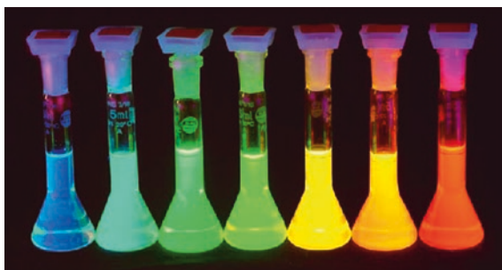
Fig. 4.10 Emission colors of ZnS-capped CdSe QDs excited with a near UV lamp (Credit Image courtesy by http://ffden-2.phys.uaf.edu/211_fall2004.web.dir/jason_turnquist/main.htm , Access date 28 Apr 2014)
