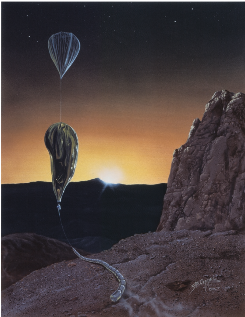
Early Mars balloon probes called for a pressurized helium balloon at the top with a Montgolfier solar-heated balloon below (© Michael Carroll/Planetary Society)
