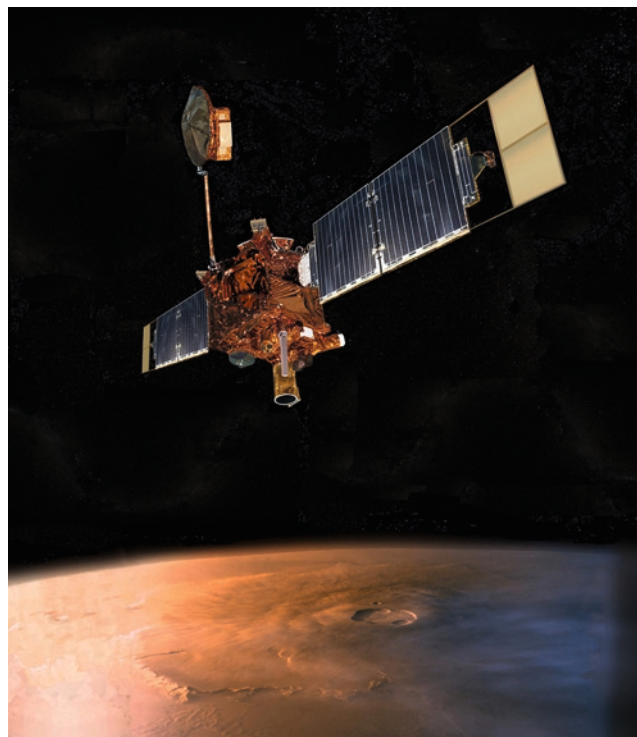
Mars Global Surveyor used its solar panels as air brakes to circularize its orbit (Corby Waste, JPL)
