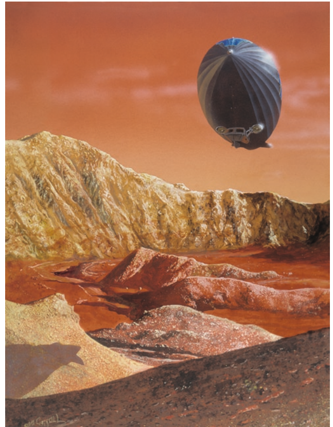
Piloted dirigibles might be possible, even in the thin Martian air. Here, an MIT study envisions an airship with a black gas envelope to utilize solar heating of the gases inside. Note the solar cells on top for power, and the large turbines to move the craft in Mars' 7 mbar pressure (© Michael Carroll)
