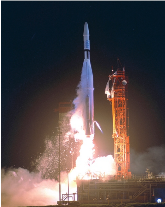
Launch of Mariner 1 on an Atlas Agena 5 booster. The craft went off course and had to be destroyed by the Range Safety Officer less than 5 min after liftoff (NASA)
