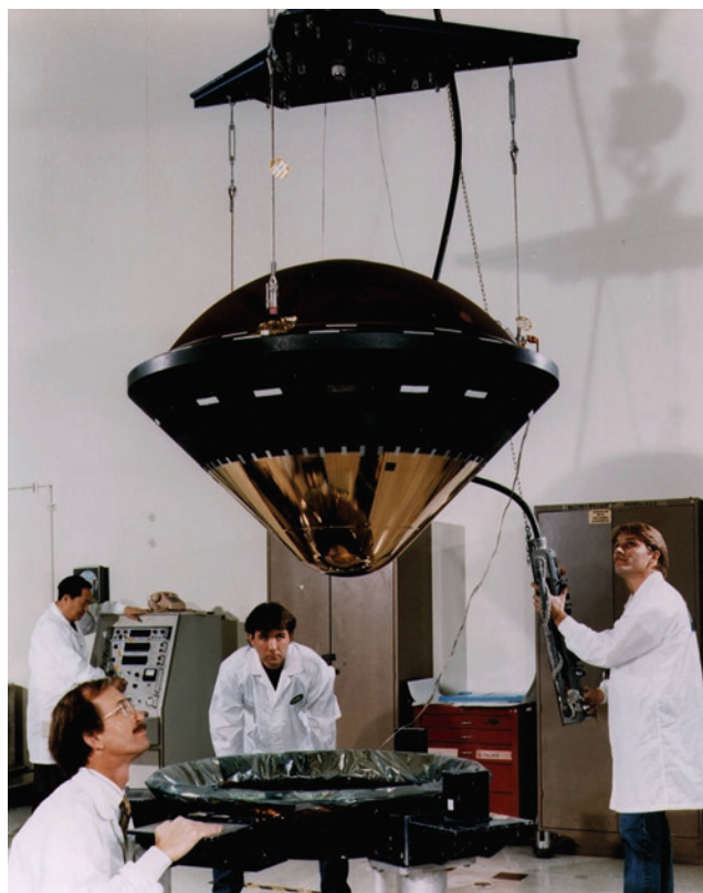
Galileo rested within a carbon phenolic heat shield that could survive temperatures hotter than the surface of the Sun (NASA/JPL)
