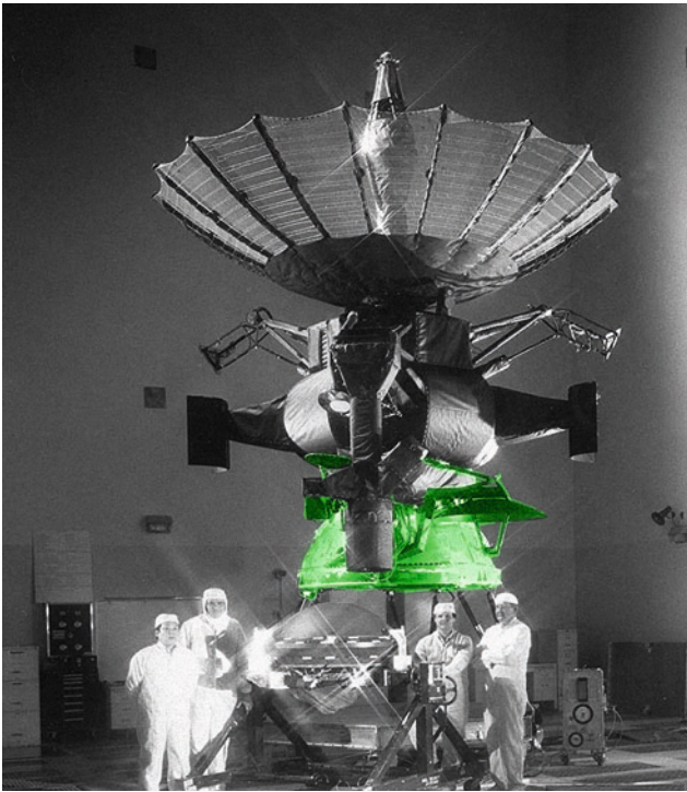
Galileo being assembled in the clean room at JPL. The despun section is in green (NASA/JPL)
