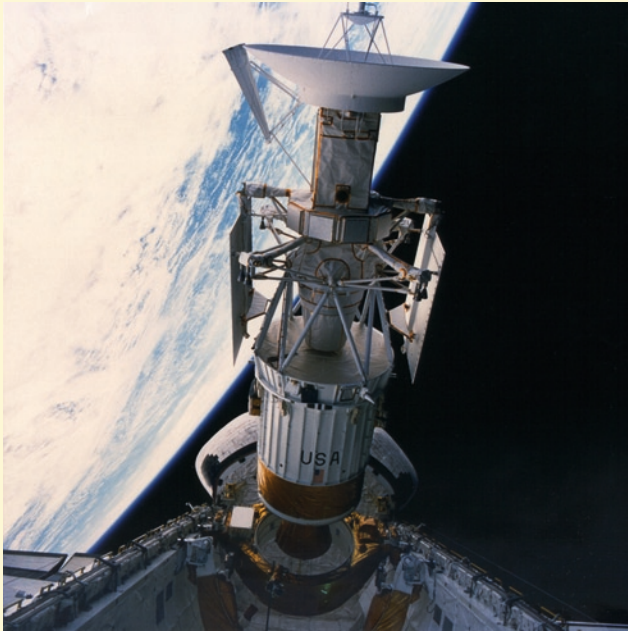
The Magellan Venus orbiter was the first spacecraft to use aerobraking for a prolonged period. Its solar panels, seen here folded at its sides prior to deployment from the shuttle Atlantis's cargo bay, served as aerodynamic brakes in Venus's thin upper atmosphere (NASA)
