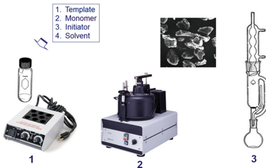
Fig. 3 A classical process for preparing MIP particles: 1 Dissolution of reagents in solvent followed by crosslinking polymerization, 2 mechanical grinding, 3 solvent extraction to remove the molecular template
