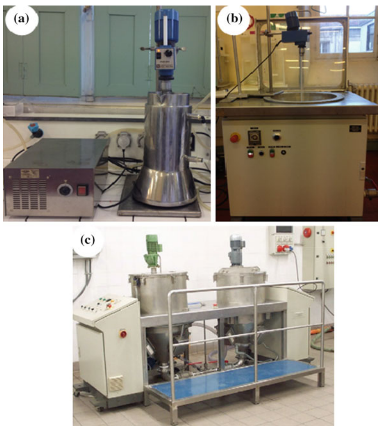
Fig. 3.4 Industrial ultrasound apparatus: a 3 L, b 30 L, c 300 L
