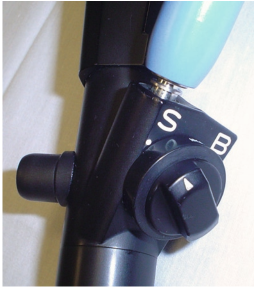
Fig. 2. Pentax instrument. The suction channel for the endoscope is different from that of the balloon and the knob has to be manually switched from scope ( S ) position to balloon ( B ) as desired.
