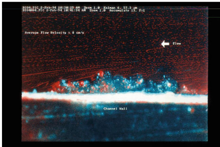
Fig. 5 Confocal side view of a biofilm using particle image velocimetry to reveal the fluid pathlines around the biofilm. The average flow velocity was 8 \text{ cm s}^{-1} . The flow over and around the biofilm imparts a shear stress over the surface, downstream drag and the aerofoil effect creates lift
