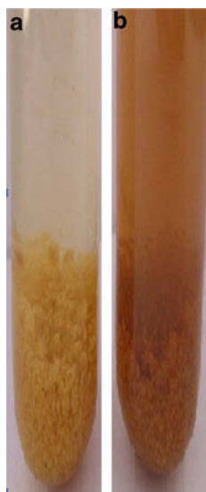
Fig. 1: Pictures show the color changes (a) before and (b) after the process of reduction of \text{Ag}^+ to Ag nanoparticles
