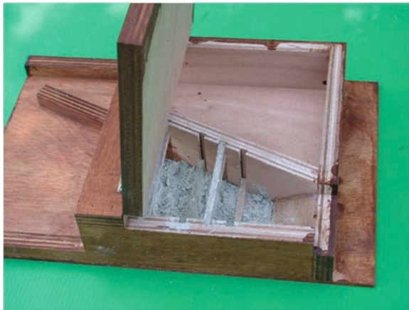
Figure 5. ‘Triwax’ dispenser for disseminating biological agent via honeybees. The left-hand side of the device is inserted into the hive and foragers exiting the hive are dusted with the powder.
