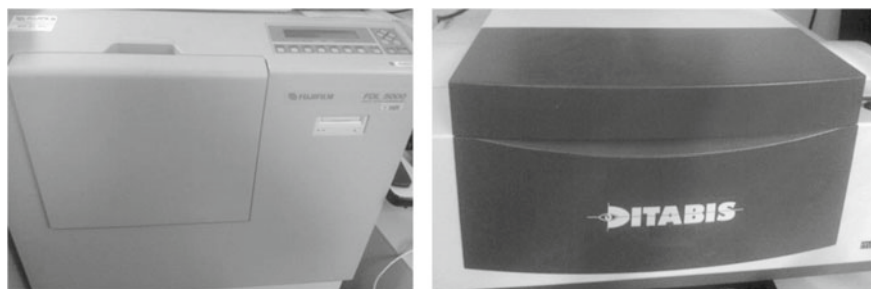
Fig. 13 Photo pictures of the scanners for imaging plates made by Fuji (left panel; 3760 \times 3000 pixels and 16 bit dynamic range) and Ditabis (right panel; 5744 \times 5066 pixels and 20 bit dynamic range)
