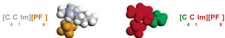
Fig. 5 [C_4C_1Im][PF_6] ; (left) Corey, Pauling, Koltun (CPK) colours; (right) red for polar domains, i.e. the imidazolium ring of the cation and the PF_6^- anion, and green for nonpolar domains, i.e. the side chain of the imidazolium [34]
