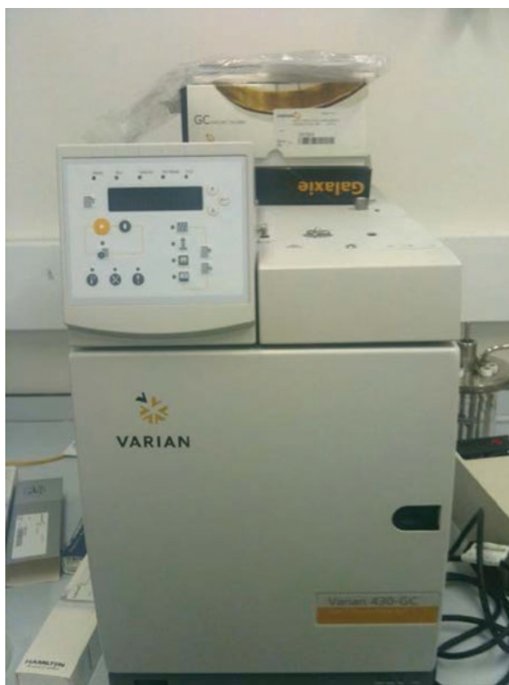
Fig. 2.3 Photograph of the gas chromatograph unit used during photocatalysis experiments
