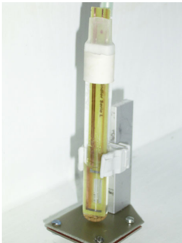
Fig. 6.3 Miniature cell for electrode stripes like shown in Fig. 6.2. For Explanation, see text
