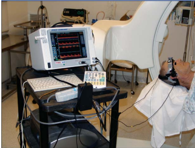
FIGURE 14-3. The typical setup during transcranial Doppler monitoring in the angiographic suite. The patient is placed in a supine position and the transcranial Doppler bracket is fixed to the head prior to baseline angiography.
