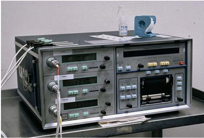
FIGURE 45-1. Novametrix 800 tcpO 2 monitor with three modified Clark electrodes.
