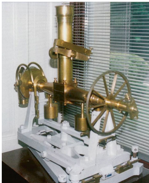
Fig. 3.77 One of the Stackpoole broken-tube transit telescopes used by the Americans (U.S. Naval Observatory; photograph by the second author)
