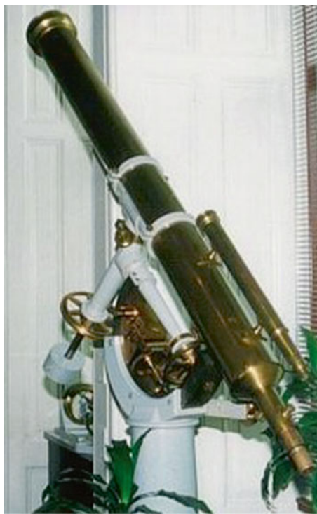
Fig. 3.76 One of the 5-in. equatorially-mounted Clark refractors used by the Americans (U.S. Naval Observatory; photograph by the second author)
