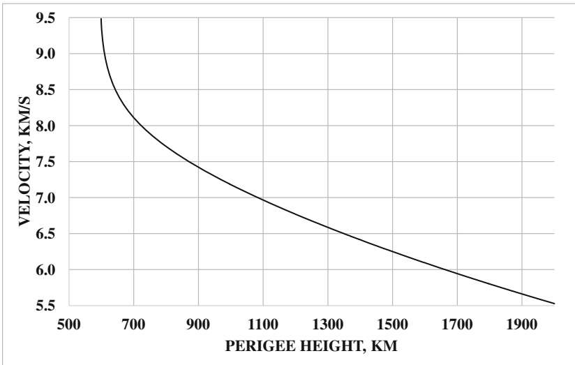
Fig. 3. Velocity of satellite projection movement to the day surface in the orbit perigee as the function of perigee height h_\pi .
