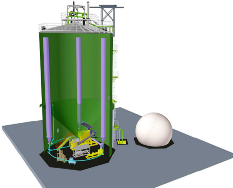
Fig. 7.15 Sectional view of a Dranco digester showing internal feeding tubes and the feeding pump under the digestion tank (photo courtesy: Organic waste systems n.v.)
