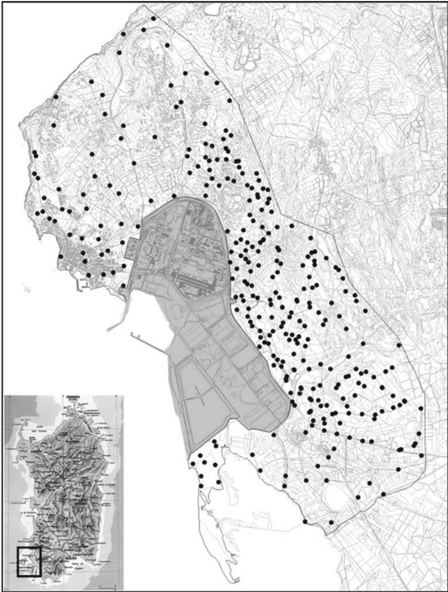
Fig. 7.2 The Portosucos Municipality potentially contaminated area: sampling points of the investigation plan [5]
