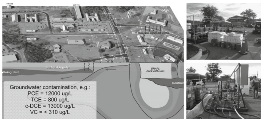
Fig. 15.3 Field demonstration of ISCO for remediation of chlorinated solvent contaminated groundwater using co-injection of oxidant and amendments to enhance delivery (from Crimi et al. [10]). The ISCO system includes co-injection of \text{KMnO}_4 (5 g/L), SHMP (5 g/L), and Xanthan gum (0.5 g/L) during a single well injection event to treat a 10m diameter zone of sand and silty sand in the depth interval of 11 to 16m below ground surface
