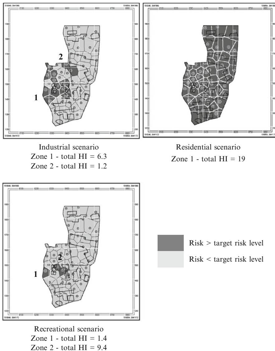
Fig. 5.3 Non-cancer risk zones with total HI > 1 under the industrial (adult receptor), residential (child receptor) and recreational (child receptor) scenarios for the Moni site, Cyprus
