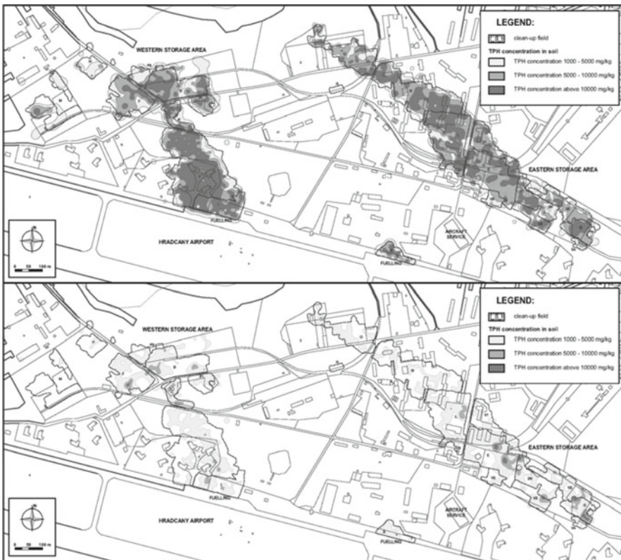
Fig. 21.1 Site Layout with Soil Contamination Extent – Initial (1997) and Closure (2009) Conditions
