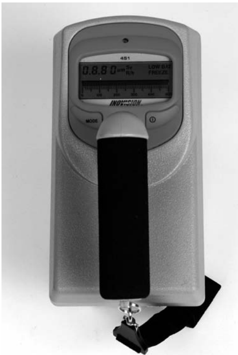
Figure 4. A portable ionization chamber survey meter (Cardinal Health; Invision, Model 451). The display shows the features during the initial check phase immediately after turning on the instrument.
