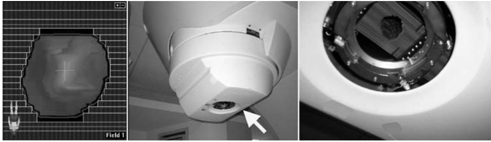
Figure 5. Beam's eye view showing target shape. Instead of constructing a custom block for the conformal shape of the target, at left a MLC (narrow rectangles) approximates the shape of the conformal beam. Each rectangle represents a tungsten leaf which moves left and right across the field of view shown under computer control. In this example, the MLC leaves would remain stationary while the treatment beam is on, providing a dose distribution very similar to a custom block. At center, the position of the MLC (arrow) on the linac gantry is shown; X rays emerge from the MLC-shaped aperture. At right, close-up photograph of the actual MLC, whose leaves are shaped to the field shown in the left image.
