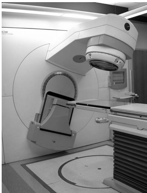
Figure 1. Photograph of an isocentric medical electron linear accelerator (Elekta Precise, Elekta Inc.).
