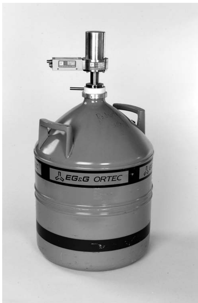
Figure 19. Left Panel: liquid nitrogen dewar (left; Ortec, Model unknown) for cooling a germanium detector (right; Princeton Gamma Tech, Model RG-11B/C); Right Panel: The assembled detector ready for use.
