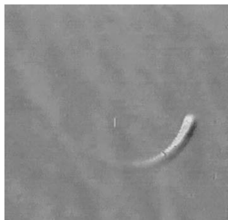
Figure 5. Micrograph of 1 \mu\text{m} bead being manipulated in a circle with an optical tweezers device. The comet tail is the result of the bead moving faster than the video frame rate.
