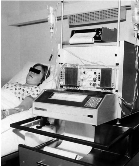
Figure 1. Biostator is the first commercial artificial endocrine pancreas. (Courtesy of Dr. Freckmann, Institute for Diabetes Technology, Ulm, Germany.)
