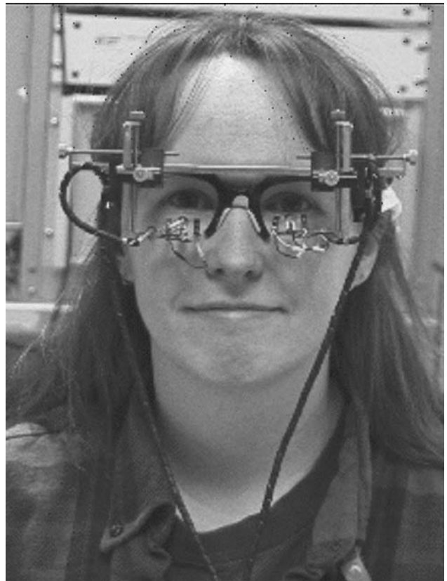
Figure 3. IR system to measure the horizontal eye movements of both eyes shown mounted on an earth-fixed frame (a) and spectacle frame (b) for human subjects and on a spectacle frame for a canine subject (c).
