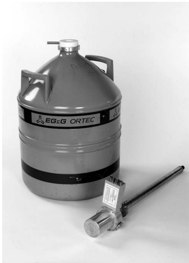
Figure 19. Left Panel: liquid nitrogen dewar (left; Ortec, Model unknown) for cooling a germanium detector (right; Princeton Gamma Tech, Model RG-11B/C); Right Panel: The assembled detector ready for use.
