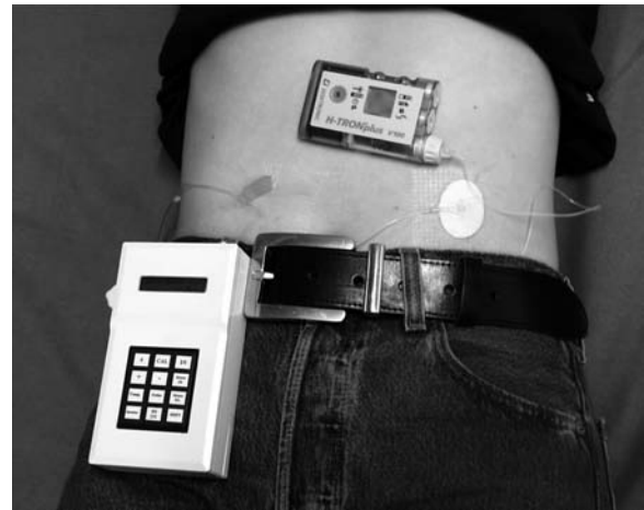
Figure 3. The system V4-IDT from the ULM group. The system uses a glucose monitor based on microdialysis integrated with a portable computer and an H-Tron pump, Disetronic. (Courtesy of Dr. Freckmann, Institute for Diabetes Technology, Ulm, Germany.)
