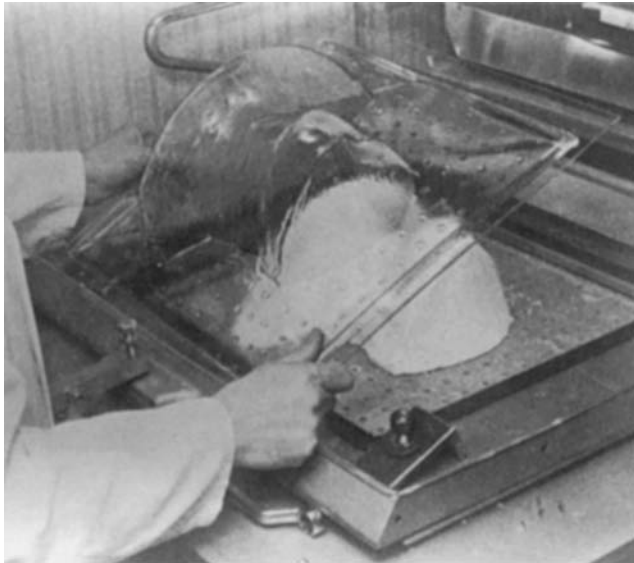
Figure 11. Plastic shell. Transparent form-fitting plastic shells fabricated using a special vacuum device. (See Ref. 11.)
