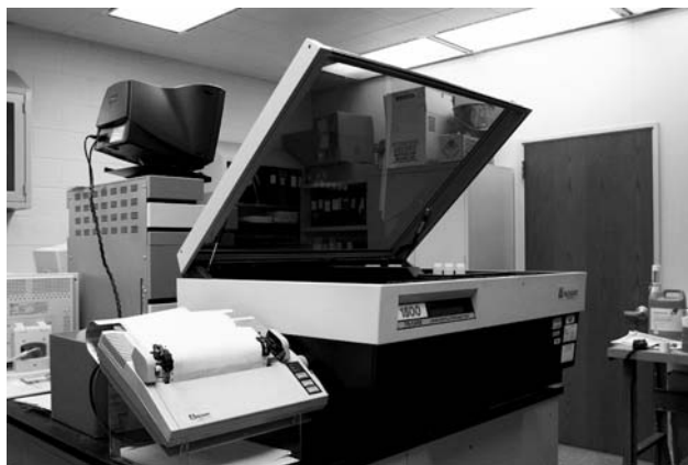
Figure 12. A liquid scintillation counter system for beta particles (Canberra; Packard, Model B1500 Tri-Carb).
