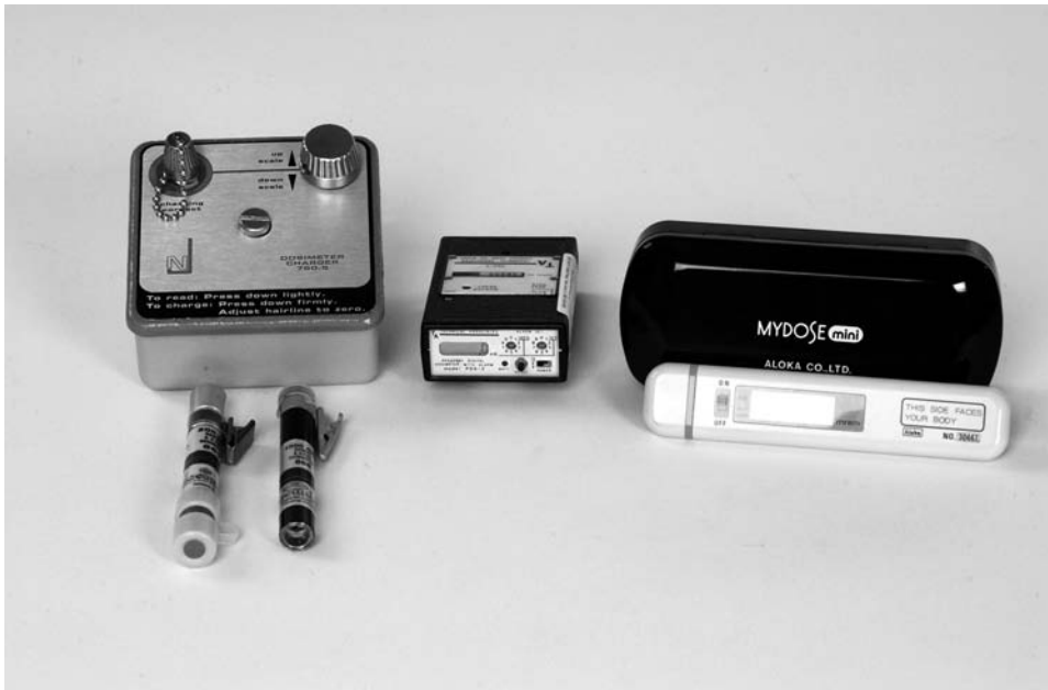
Figure 3. Personnel dosimeters. Low dose (bottom left; Dosimeter Corp., Model 862); and high dose (bottom right; Dosimeter Corp., Model 866) \gamma - and X-ray pocket dosimeters, with charger (top left; Jordan Nuclear Co, Model 750-5). An alarming personal digital dose meter (center; Technical Associates, Model PDA-2) and a miniature pocket digital dosimeter (right; Aloka Co, LTD., Model MYDOSE-mini).
