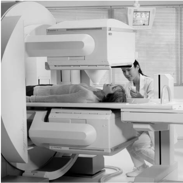
Figure 10. Dual-headed gamma camera. Both detector heads are mounted on the same gantry to allow translation (for whole body) and rotation (for SPECT) of the system. An open geometry permits use of gurneys with this system.
