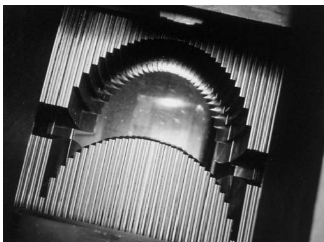
Figure 29. Multileaf Collimation (MLC) system. Computer controlled system used to shape beam aperture and also to deliver IMRT. (Courtesy of Elekta AB.)
