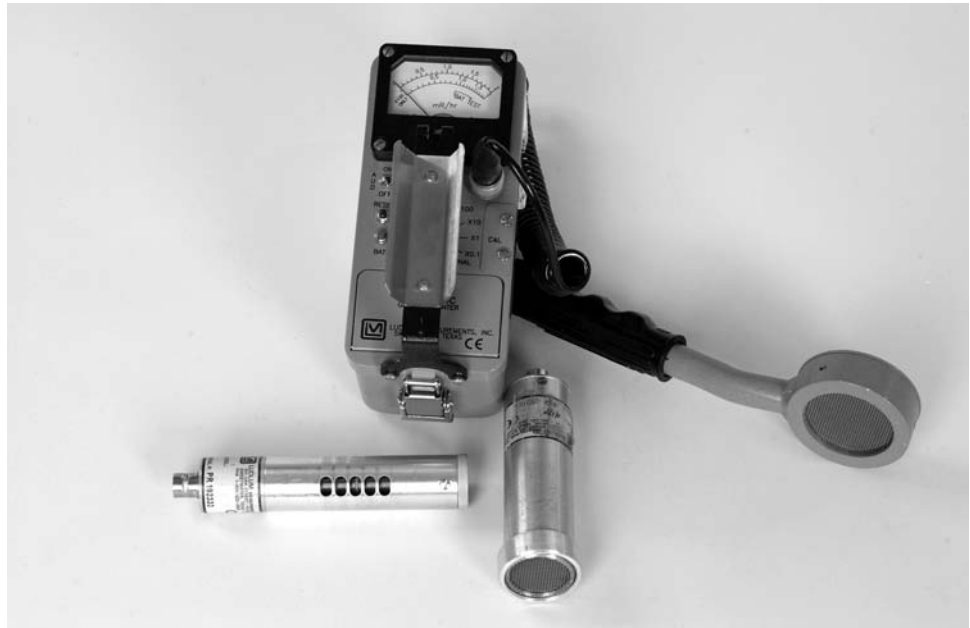
Figure 8. Portable GM counter (top; Ludlum Measurements, Inc. Model 14C) with an open side-window probe (left; Ludlum Measurements, Inc. Model 44-38), an end thin-window probe (center; Ludlum Measurements, Inc., Model 44-7), and a pancake probe (right; Ludlum Measurements, Inc., Model 44-9).
