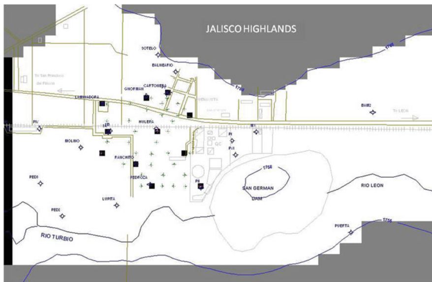
Fig. 6 Design of the capture zone. The crossed circles indicates the water table monitoring point (hydraulic head must be located up the aquifer bottom )
