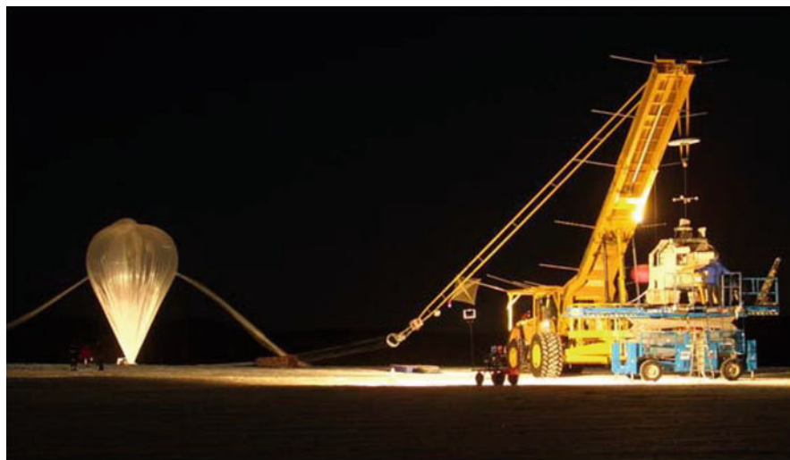
Fig. 10.24 TELIS-MIPAS launch at Esrangle, Sweden; March 2009. Balloon size: 400,000\text{ m}^3 ; payload weight: 1,200 kg
