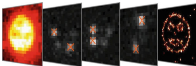
Fig. 6 Localization-based super-resolution microscopy: diffraction-limited TIRF image of 1.5 \mu\text{m} smiley ( left ) produced by single-molecule cut-and-paste [52]. Selection of 3 of 8,000 camera images used for reconstruction of the artificial super-resolution image ( right )
