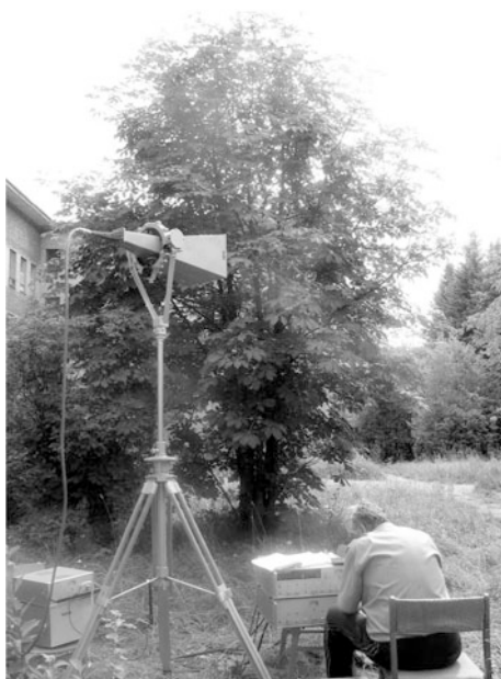
Figure 8.8. In situ measurement of electromagnetic wave attenuation by vegetation canopies in the 100–1,000 MHz frequency band.
