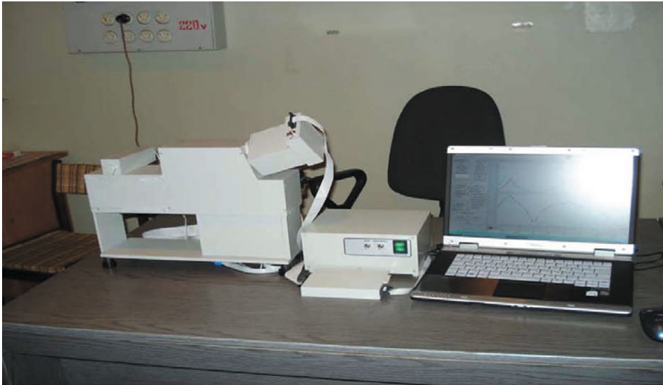
Figure 6.23. General view of the multi-channel spectropolarimetric system (Soldatov, 2011).
