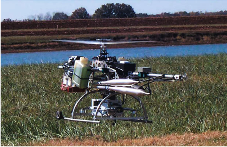
Figure 1.31. The Microwave Autonomous Copter System (MACS) unmanned aerial vehicle (UAV), a helicopter equipped with a 6 cm radiometer, data acquisition system, GPS receiver, and power supply battery (Shutko et al. , 2010).
