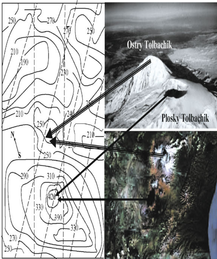
Figure 7.5. A map of the distribution of radiobrightness temperature T_j near the Gt. Tolbachik volcano in Kamchatka by means of the IL-18 flying laboratory at wavelength \lambda = 27 cm. This map was reconstructed by means of GIMS technology based on trace data.
