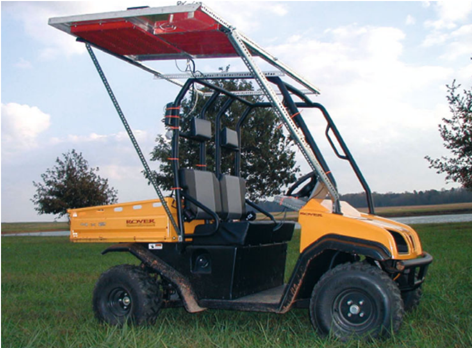
Figure 1.29. General view of the manned rover-type mobile platform equipped with three portable microwave radiometers, operating at wavelengths 6 cm, 18 cm, and 21 cm. Also equipped with a folding panel of 1.5\text{ m} \times 1.5\text{ m} for instrumentation installation along with a GPS receiver, data acquisition system, and power supply battery (Shutko et al. , 2010).
