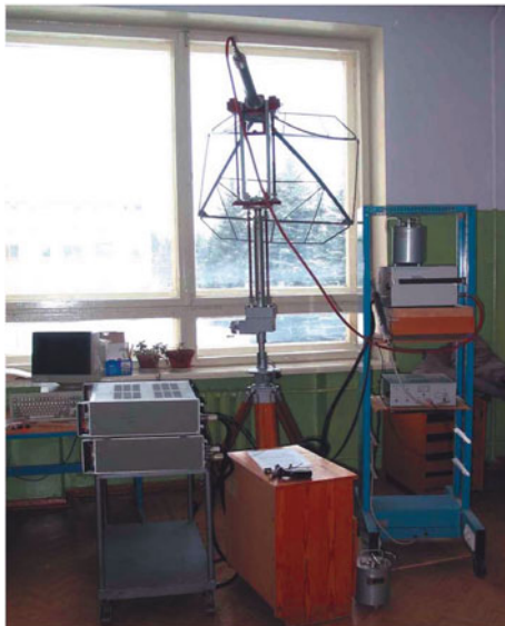
Figure 8.7. Measuring system used to assess electromagnetic wave attenuation in in situ experiments (Chukhlantsev, 2006).
