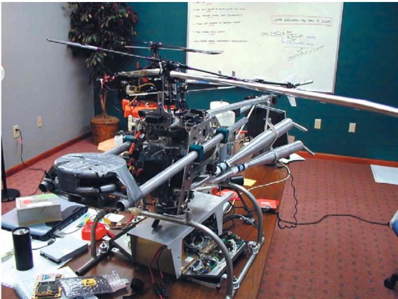
Figure 1.32. Installation procedure for the unmanned helicopter's on-board radiometer.
