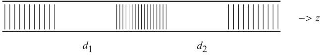
Fig. 18 Sketch of a resonant cavity formed by two standard Bragg gratings at either end, into which the PT -symmetric grating with index profile e^{2i\beta z} is inserted. The highly-selective right reflectivity of the PT -grating can serve to eliminate competing modes of the original cavity
