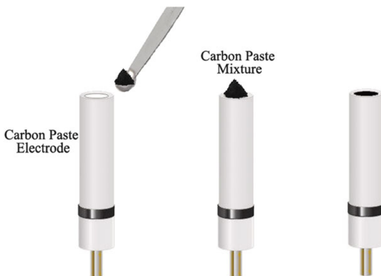
Fig. 4.12 Preparation of carbon paste disc electrodes [Reprinted with permission from BAS Inc.]
