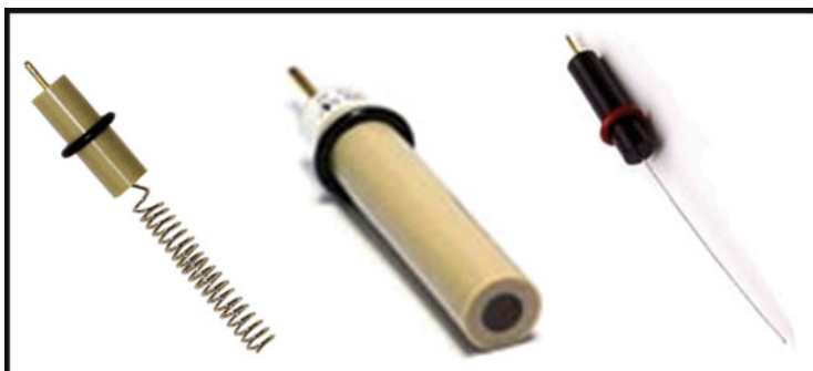
Fig. 4.3 Pt electrode different geometries [Reprinted with permission from BAS Inc.]
