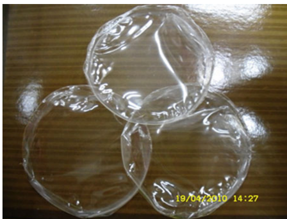
Fig. 3 Film of thermoplastic starch detached from its mold once the drying process is finished
