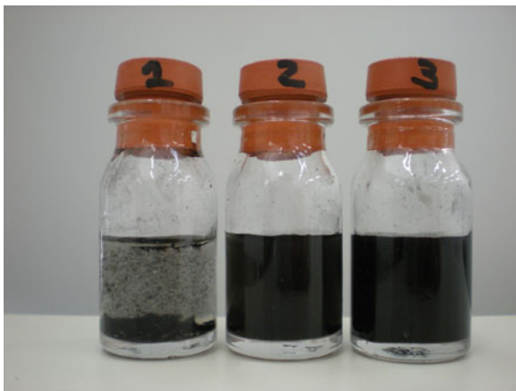
Fig. 3 Aqueous dispersion of carbon nanotubes 2 hours after sonication in an ultrasonic bath, (1) pristine MWCNT; (2) MWCNT functionalized with carboxylic groups; (3) MWCNT functionalized with hydroxyl groups
