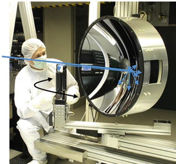
Fig. 14.8 Roughness characterization of an EUV collector mirror substrate by light scattering measurements performed by the first author of this chapter
