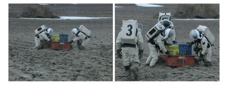
The trailer with the 130 kg of equipment sank in the mud and could not be pulled out by two or four people with muddy and wet EVA suits. *Credit* Discovery Channel
