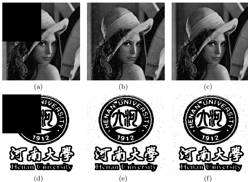
Fig. 1. The experimental result images under the different attacks. (a)(d) The cropping 1/4 of the experimental result image. (b)(e) Affected with pepper and salt noise. (c)(f) Affected with Gaussian noise.
