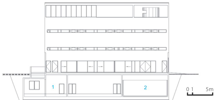
Section 1: 剖面图1: 1. Drinking water room 1. 直饮水机房 2. Interior fire pool 2. 室内消防水池
